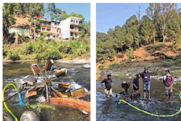
Testing of water lifting device at Kosi river bed
