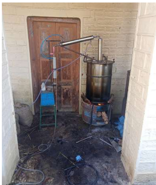
Fig. 6.5.2. Small scale steam distillation unit for extraction of essential oil from pine needle
